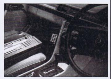
The fax machine is now moving out of the office with the introduction of the NEC Carfax Cellular Line Interface. This not only allows a fax to be sent via the cellular network but also provides a connection means for portable computers.
